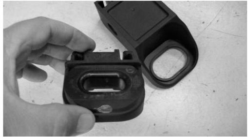
22. Remove rubbers from original radiator mounts also remove the metal ring from inside the rubber and fit the rubber only onto the supplied ramjet radiator mounts, the rubbers need to be fitted upside down from standard
