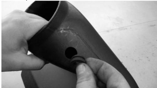
14. Insert the grommet that was removed from bottom of standard air box into the drilled hole
