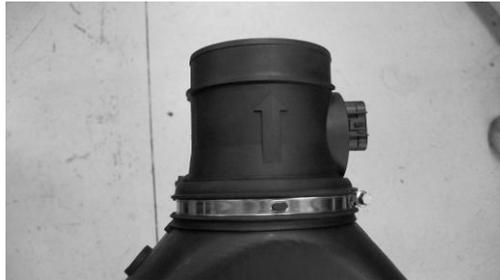
16. Fit rubber removed from stock air box onto Ramjet, then fit airflow meter (MAF) into rubber, note, this may require some lubricant, make sure arrow points towards engine
