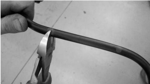
15. Cut a straight piece (50mm long) from the stock air tube that was removed. This will be inserted into the grommet hole.
