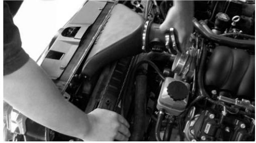
18. Once the Ramjet has been mounted between radiator and front panel secure the clamp between MAF and throttle body
