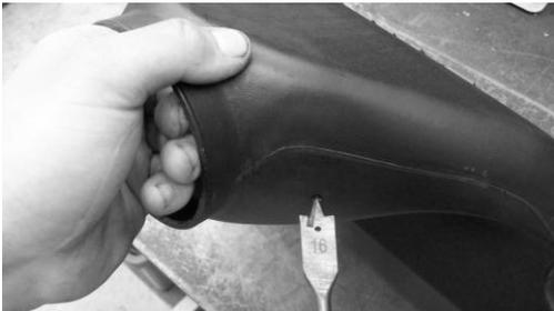
13. Drill hole using a 16mm spade bit for air vent tube as per image
