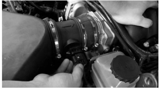
20. Plug the MAF plug wiring back onto MAF
