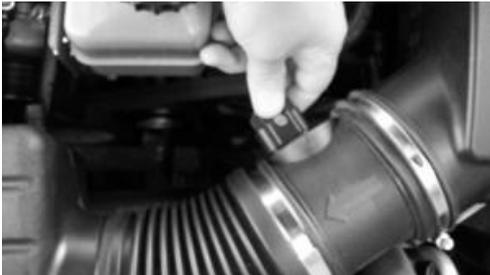
3. Unplug the airflow meter (MAF) plug from the airflow meter
