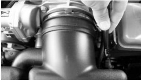
1. Remove the plastic air tube that runs from the driver's side rocker cover to the standard air box. (Put tube aside for later use)
