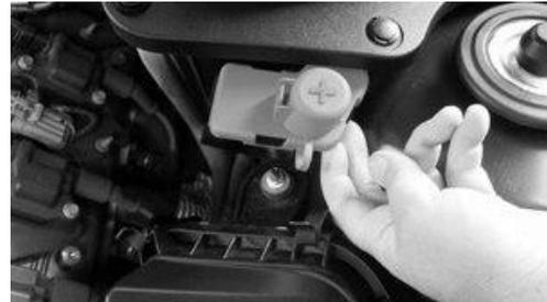
4. Remove the red cap from the positive battery terminal plug on the passenger side strut tower
