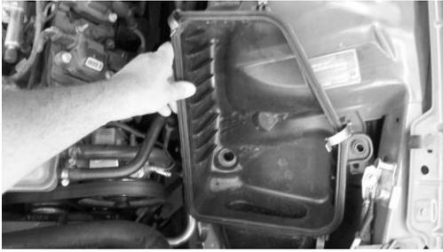
7. Remove the air box base, also remove the rubber grommet from the air box base as this will be used later on the Ramjet, you can now replace the red battery terminal cover
