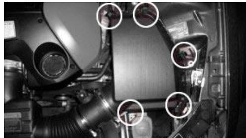
6. Unclip the 5 clips on the stock air box lid and remove complete with air flow sensor and secondary air box. Remove the MAF and rubber for later use.
