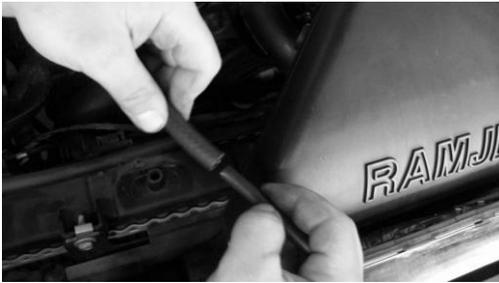
21. Insert the supplied air hose onto the driver's side rocker cover and insert the cut piece of original air hose into the other end, then push the plastic piece into the grommet in Ramjet
