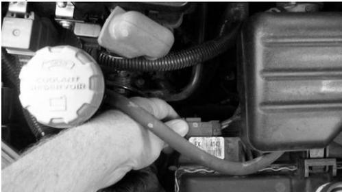
11. Remove the fan wiring plug from its bracket on the radiator, this creates more room for radiator to be tilted back
